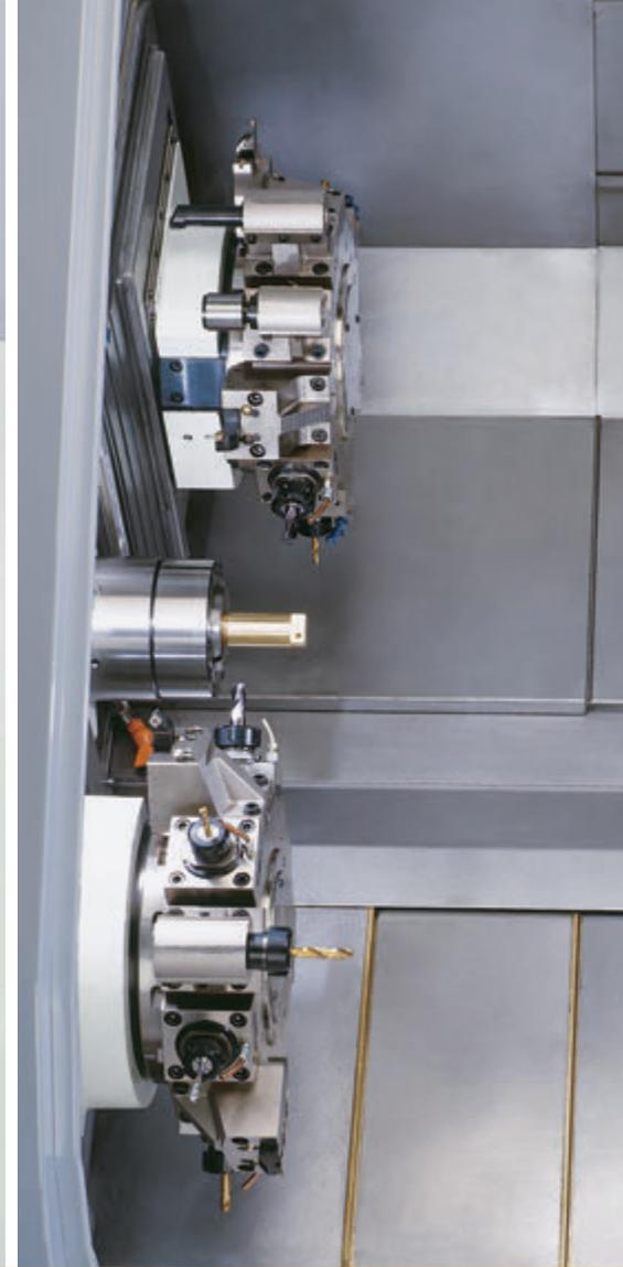
**Double-spindle turning centres featuring three turrets and three Y-axes:
