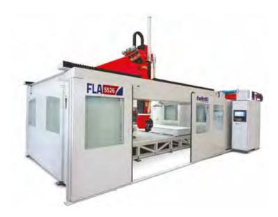
Models with Y bridge of 2600 mm and 3200 mm are made with a columns' structure that allows to achieve a high versatility in terms of sizes, maintaining an important dynamism and precision.
