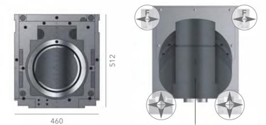
Unique ram guiding system combining accuracy and dampening capacity
