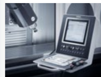
Heidenhain TNC 640 HSCI control.
