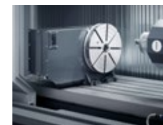
A-C axis bolt-on rotary tables (STAR 3000).
