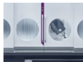
Totally encapsulated working area and safety windows.
