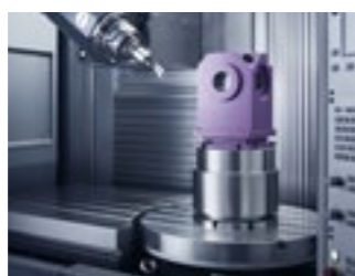
ø800 mm integrated rotary table (STAR 1500).
