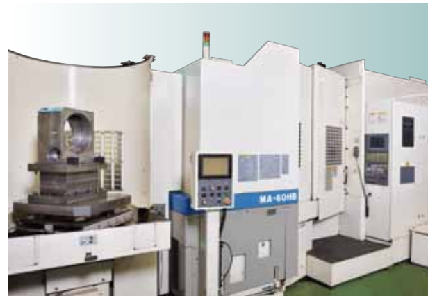
Adopting OKUMA MA-60HB HMC fro Housing machining, the parallelism and perpendicularity in boring machining can be reached 0.005mm in between spindle hole and center hole of worm shaft.
