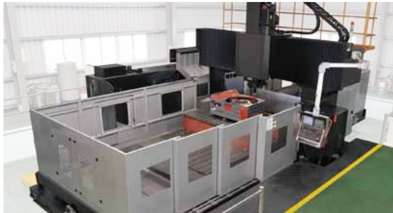
Adopting 5-Face CNC Double Column Machining Center for Large Size Housing Machining.
